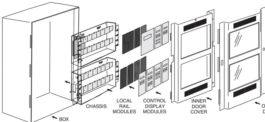
The top layer of the LRMs is referred to as the user interface layer. This layer is made up of the Main Display Interface module and a system of generic control/display modules. Any control/display module can mount on any LRM. This maximizes flexibility of design for custom systems. The inner and outer doors finish and secure the enclosure.
